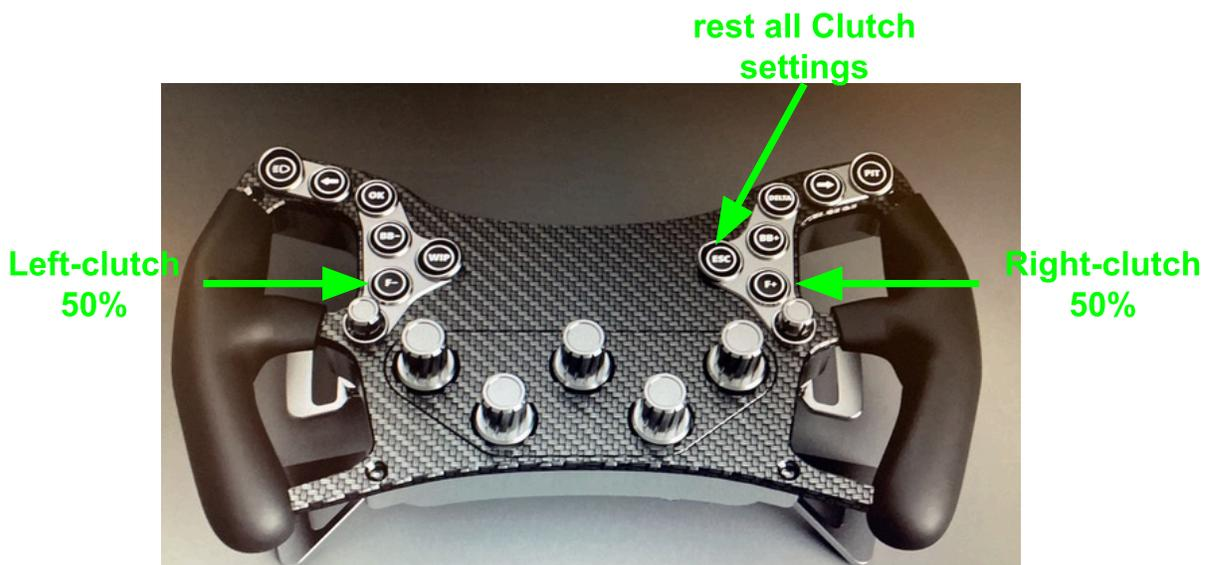
To RESET the Clutch maximum settings you can press Button 11. Thereafter you **need** to fully engage and release both Clutch-Paddles once for their re-calibration, to restore correct functionality.
